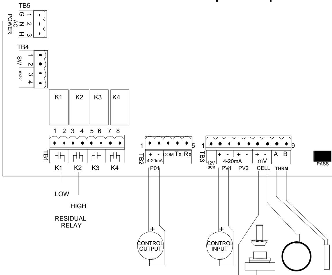
**NOTE:** ALL WIRING MUST COMPLY WITH APPLICABLE LOCAL AND NATIONAL ELECTRICAL CODES.
